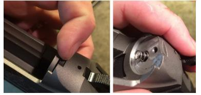
3) Remove fouling from both the firing pin channel and the threaded screw hole, as well as the face of the receiver. Breech plug cleaning brushes and solvent are excellent for this step.
