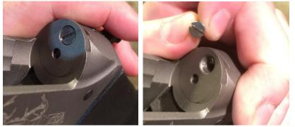
2) Using finger pressure, gently remove the bushing from the front of the frame. This should expose the Northwest firing pin and spring. Remove these and clean all four items (including the screw) using solvent and gun lube. Be mindful to remove all debris from the parts.
