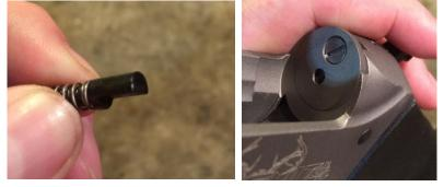
5) The hole in the top of the frame can be used for lubing the firing pin channel while shooting or in the field. However a thorough cleaning of the firing pin bushing system is necessary to maintain a well-working rifle.
