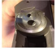
4) Replace the firing pin (with the flat cutout facing down) into the frame and push the bushing into the recess on the frame. Secure the bushing by reinstalling the screw.
